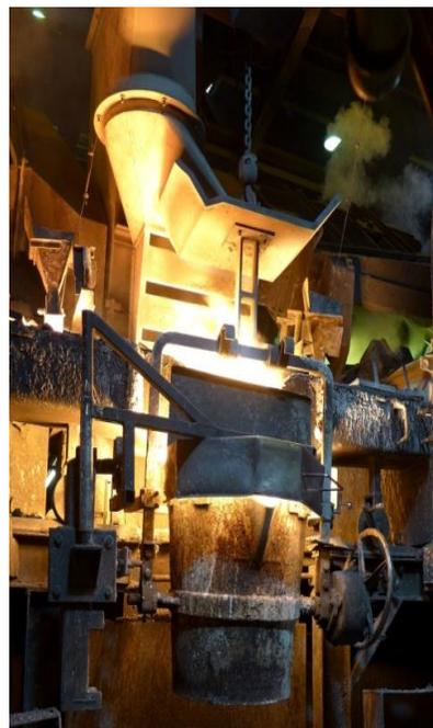
*Molten metal pouring from the electric furnace*
