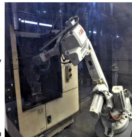
*Robots clean and remove rough edges and check the quality of the castings*
