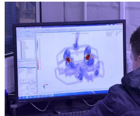
*A 3D computer simulation of the cooling characteristics of a casting*
