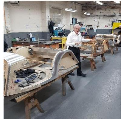
*Attaching Aluminium panels to the body frame*
